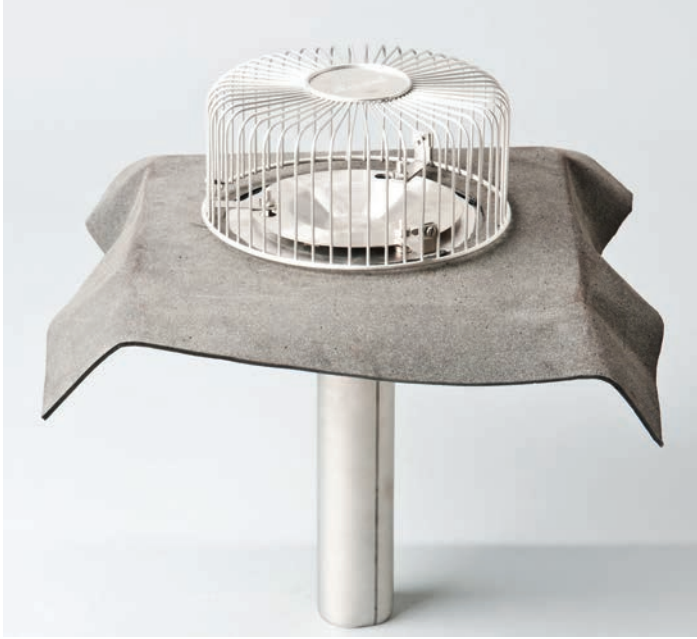
Siphonic drain made of stainless steel with bitumen collar (top) with feeder line made of bitumen, vacuum plate and pebble trap.
