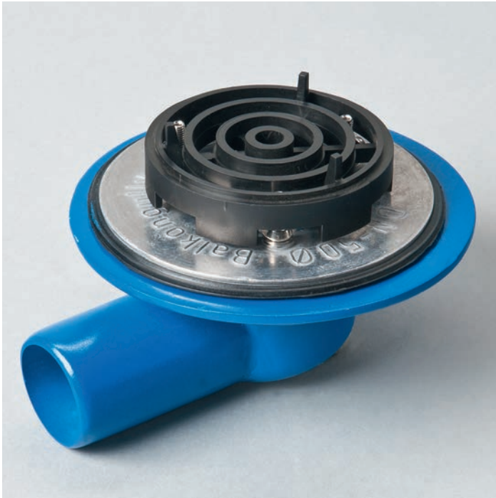
Balcony drain DN 50 with Clamp flange /with adhesive collar Balcony drains horizontal DN 50 with clamp flange and small pebble trap Balcony drains are universally deployable, fit any type of balcony and small roof. With the security clamp, any feeder line can be fitted with a flange.
